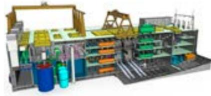
Cut away view of ThorCon 500 MW MSR power plant in ship hull. Grafik: ThorCon
